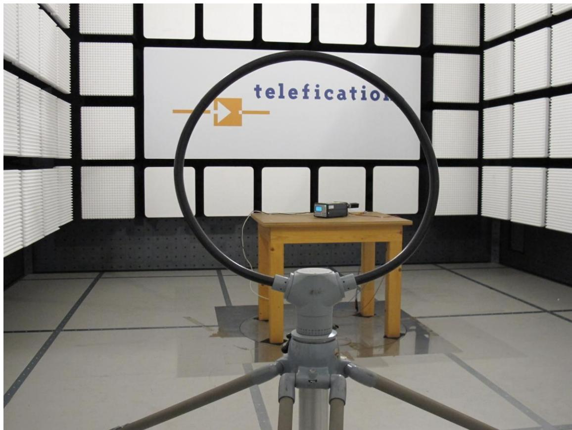
Photograph 2: *Test setup radiated emissions (0.03 - 1 GHz)*
