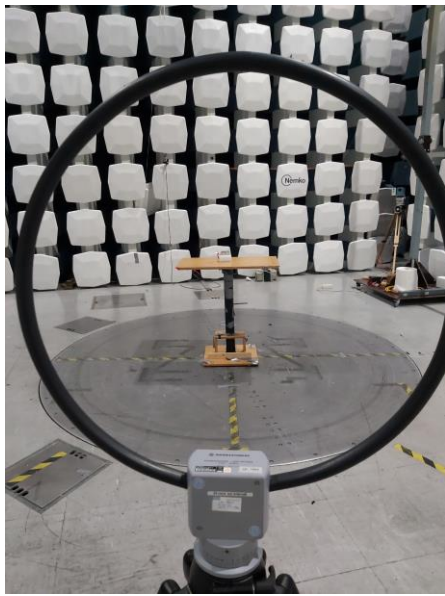
Radiated Emissions 0.009-30 MHz, Loop antenna transversal orientation
