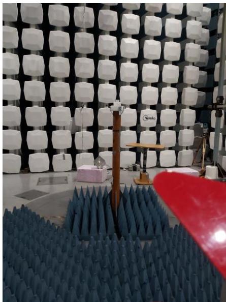
Radiated Emissions 1 – 18 GHz The EMCO 3117PA antenna is used for spurious measurements
