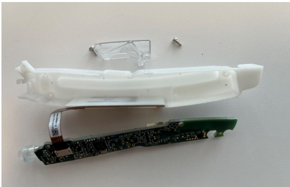
Disassembling of the RCC 1601 back side
