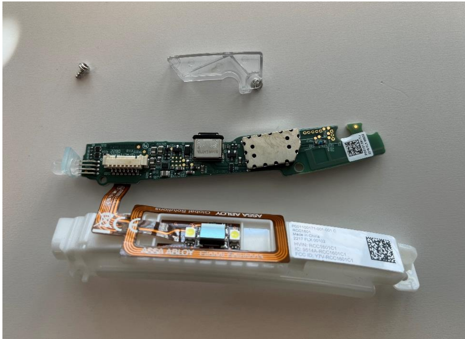
Disassembling of the RCC 1601 front side
