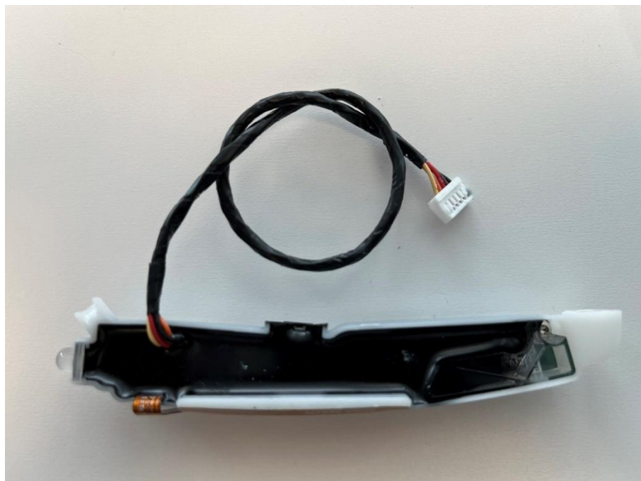
Top view of the RCC 1601 module after potting
