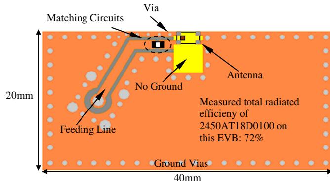
Orderable EVB p/n (comes with 1 female SMA connector mounted on the opposite side):
