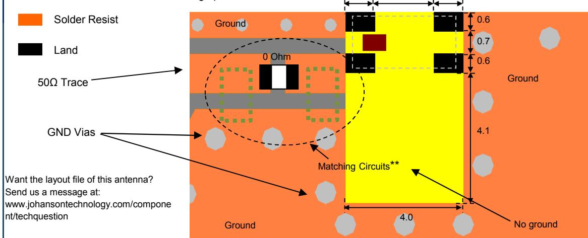
\*\*It is recommended that the designer leave available slots for a "pi" (or shunt-series-shunt) network. The antenna matching network values above are used when antenna is mounted on Johanson's evaluation board. The matching values on client's PCB will be different. Go to: <http://johansontechnology.com/tuning> and see how to obtain the new values.
