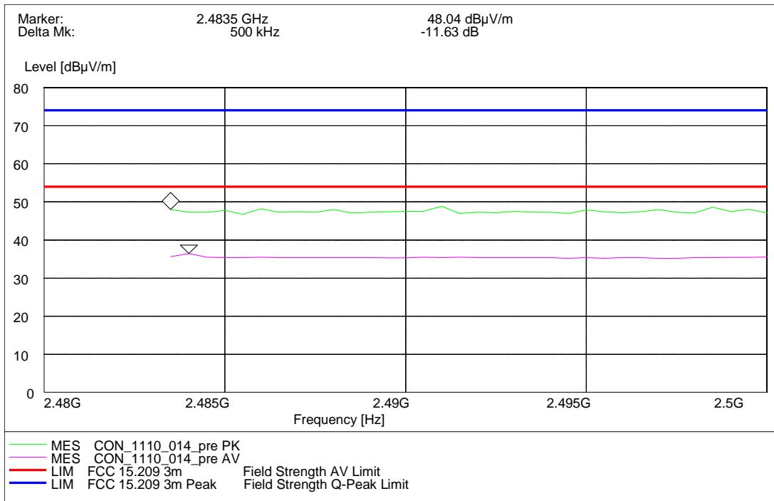
**Test: 15c.6; Frequency = 2480, Mode = BT transmit using 3 Mbps with 8DPSK modulation, Method = conducted**
