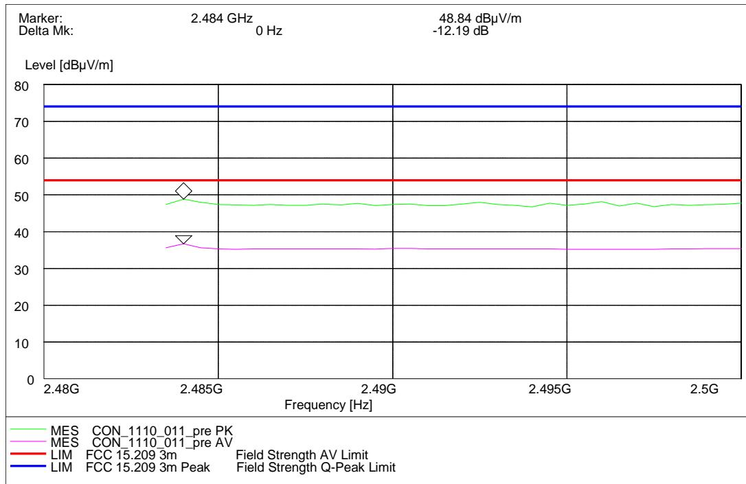
**Test: 15c.6; Frequency = 2480, Mode = BT transmit using 2 Mbps with PI/4 DQPSK modulation, Method = conducted**
