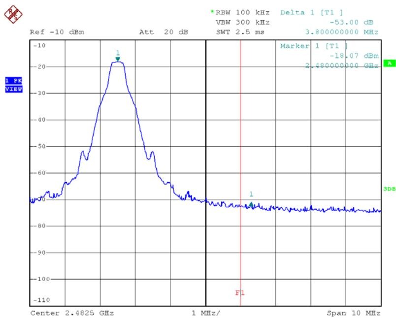
Bandedge Plot – Pursuant to FCC Part 15 Section 15. 249 / RSS-210 Section A2.9 Requirement
