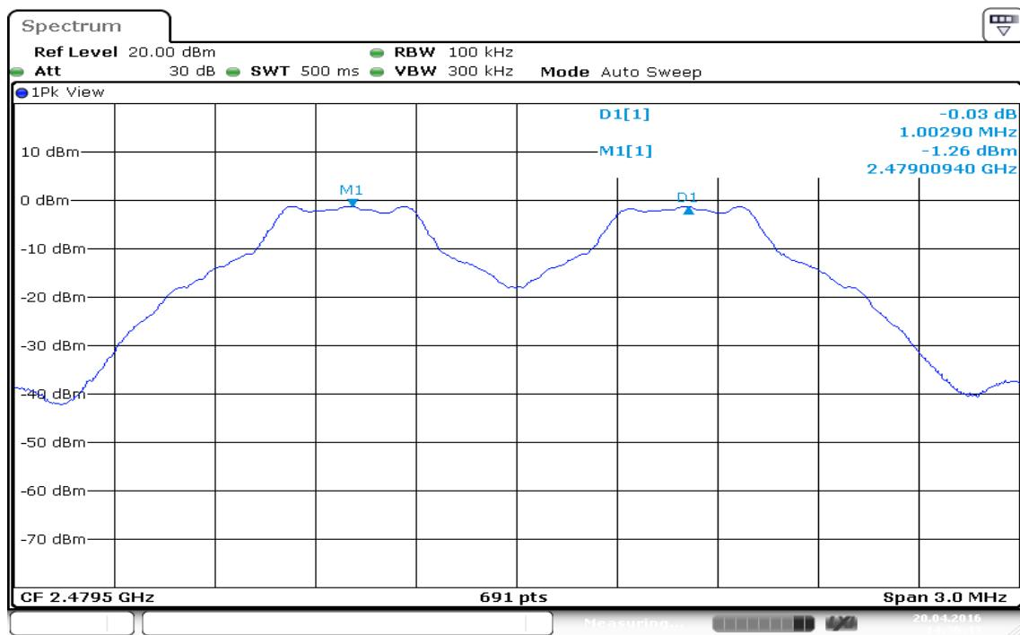
**Measurement of Channel Separation****For 8DPSK / DH5 / Low**
