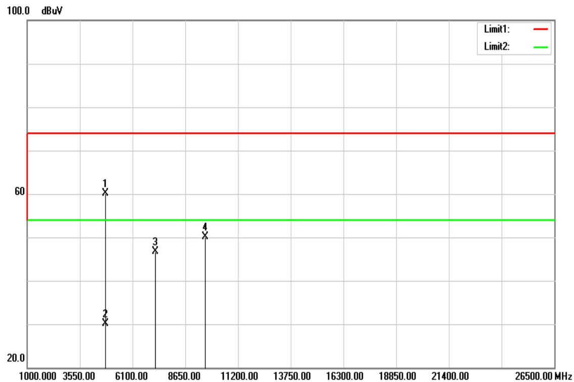
**Above 1 GHz****Operation Mode:** TX / GFSK / DH5 / CH Low**Test Date:** April 8, 2016**Temperature:** 27°C**Tested by:** Jason Lu**Humidity:** 53 % RH**Polarity:** Ver. / Hor.
