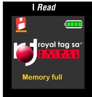
Under the disc icon, the filling rate of the memory, is graphical expressed with a progress bar.
