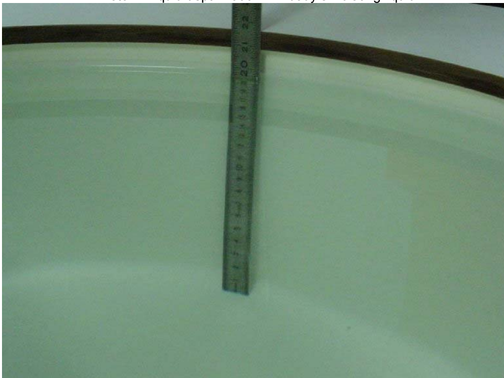
Photo 2: Liquid depth 1900 MHz body simulating liquid
