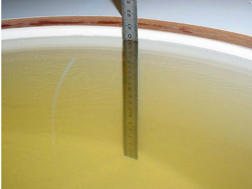
Photo 1: Liquid depth 850 MHz body simulating liquid
