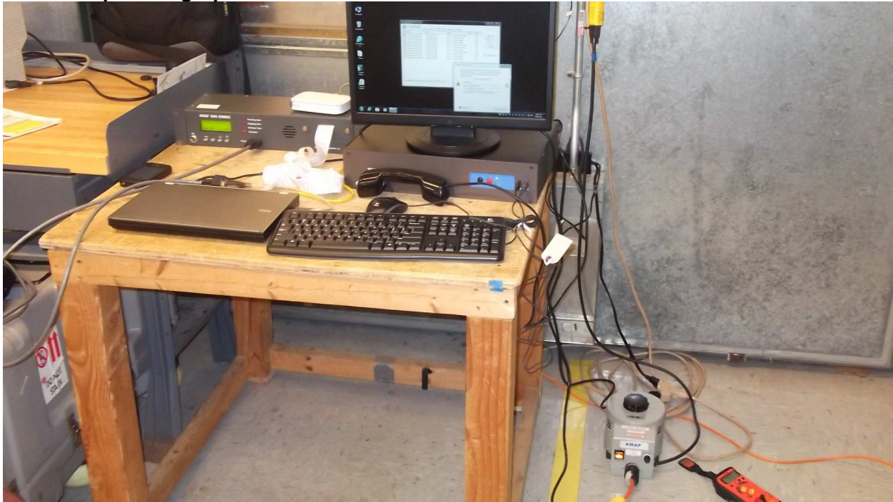
EMnet Setup with Support Encoder/Decoder and Laptop
