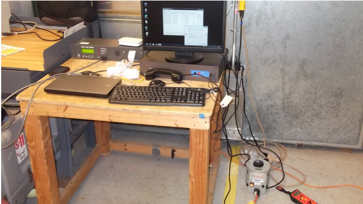
EMnet Setup with Support Encoder/Decoder and Laptop
