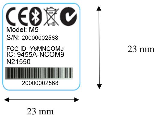
Located on the external surface of the plastic Box containing the Bluetooth PCB.
