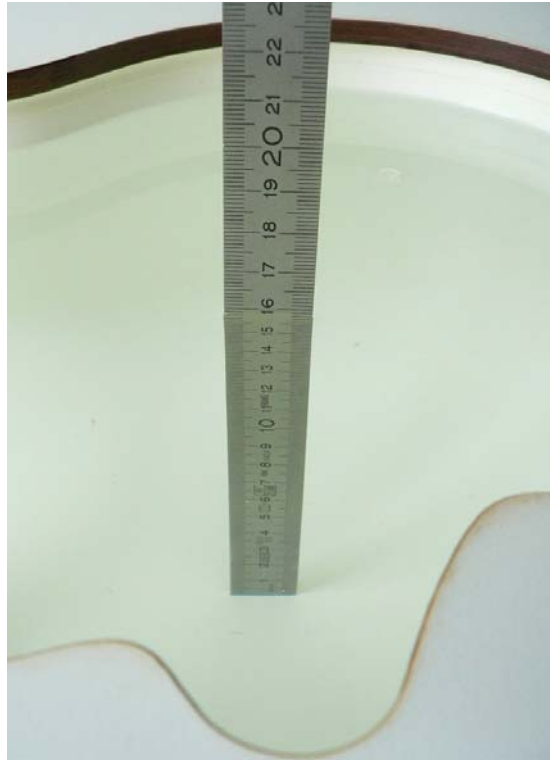
Fig. 15: Liquid depth for 2450 MHz Head measurements.
