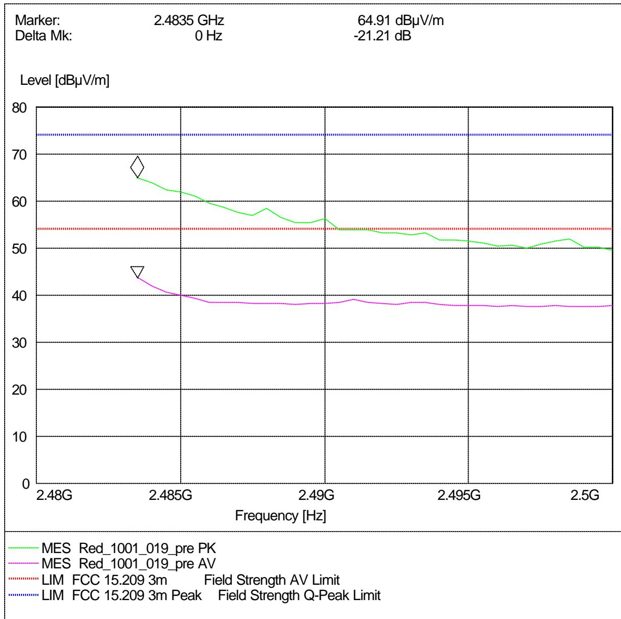
Radiated measurement (higher band edge)
