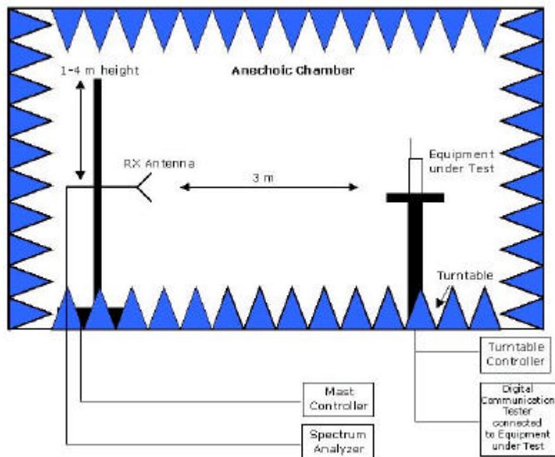
**Drawing 1:** Setup in the Anechoic chamber:
