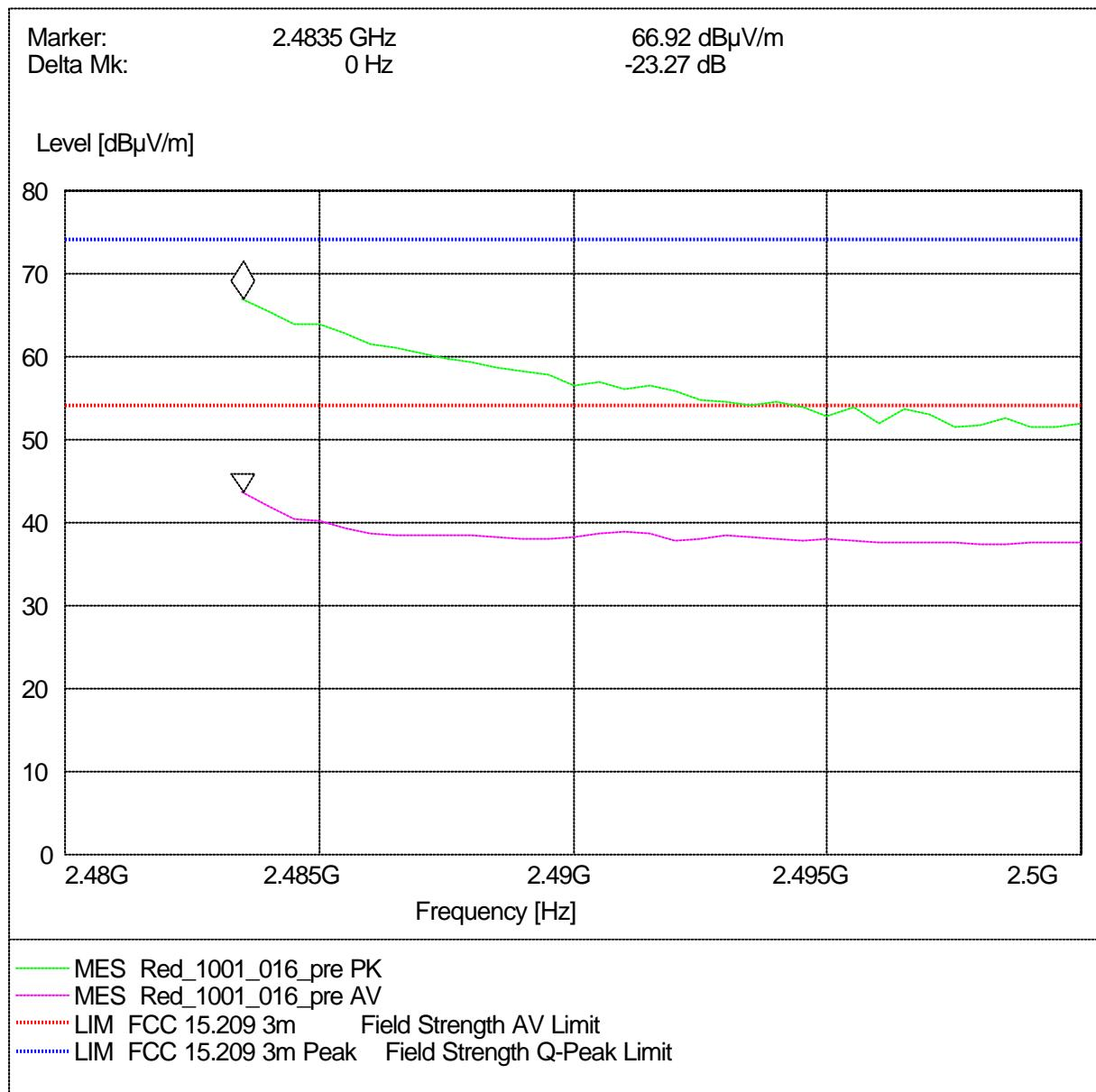
Radiated measurement (higher band edge)
