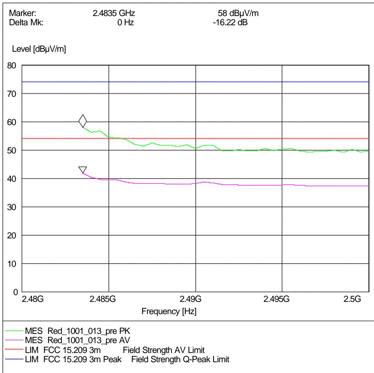
Radiated measurement (higher band edge)
