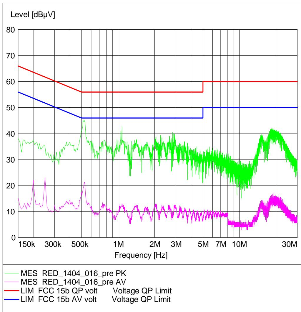
**Test: 15b.1; Mode = Powered via Laptop and generating a high power consumption**
