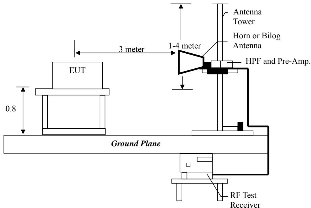
The signal is maximized through rotation and placement in the three orthogonal axes.
