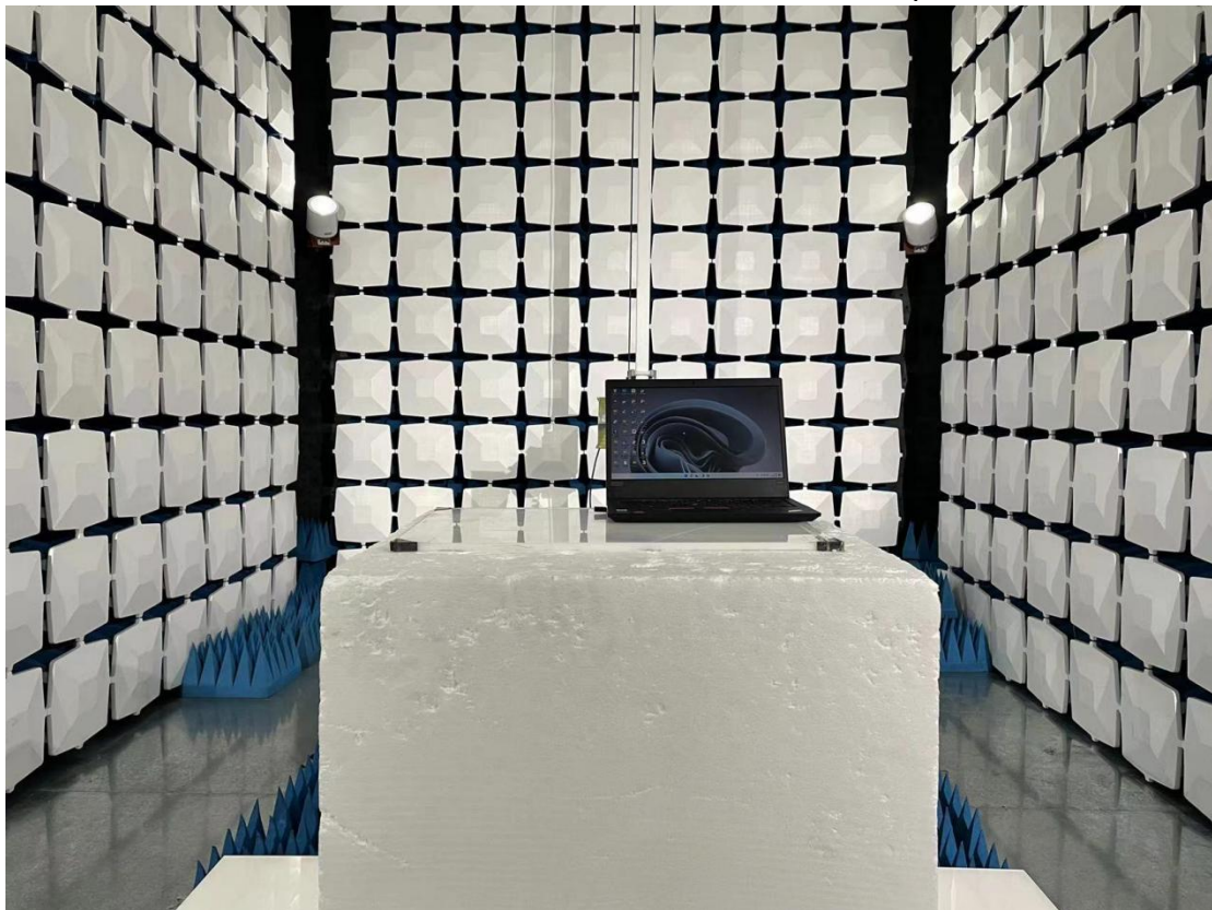
Above 1GHz for radiated emission test setup
