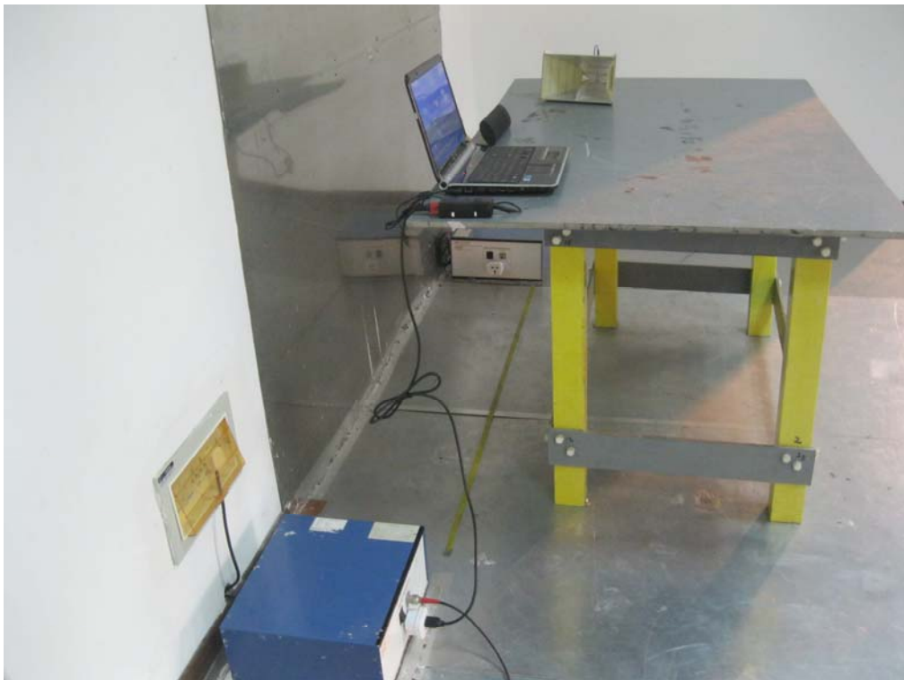
Conducted Emissions Test Setup - Side View
