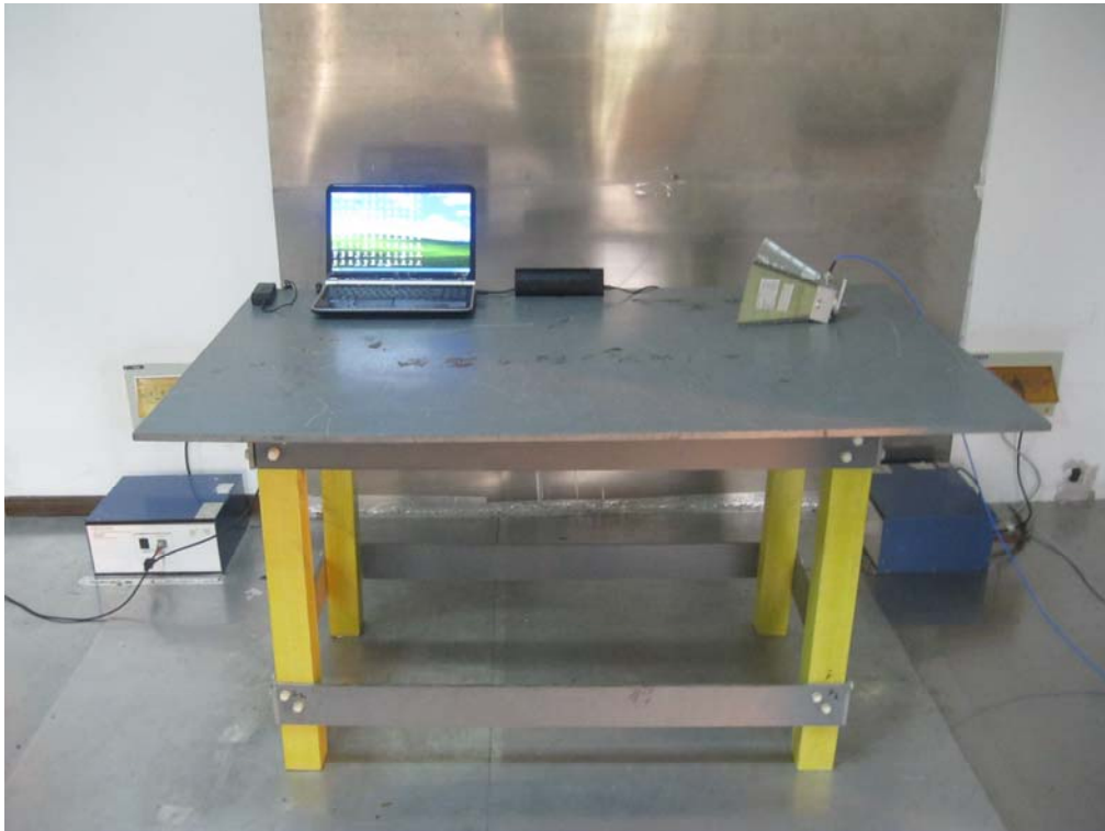
Conducted Emissions Test Setup - Front View
