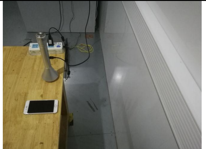
Conducted Emissions Test Setup Side View
