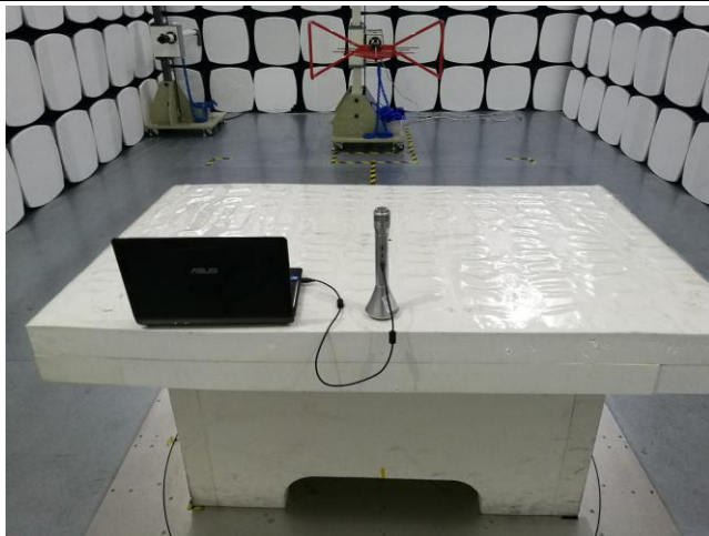
Conducted Emissions Test Setup Front View
