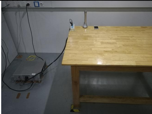
Conducted Emissions Test Setup Front View
