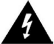
This lightning flash and arrowhead within the triangle is a warning sign alerting you of "dangerous voltage" inside the product.
