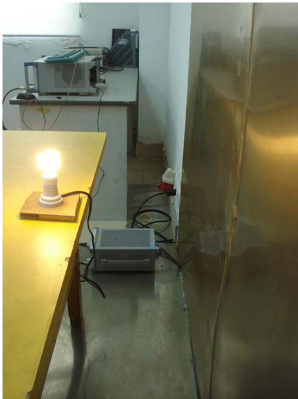
Conducted Emission Test Setup Side View
