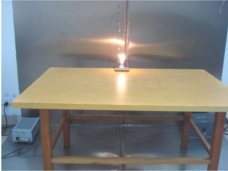
Conducted Emission Test Setup Side View
