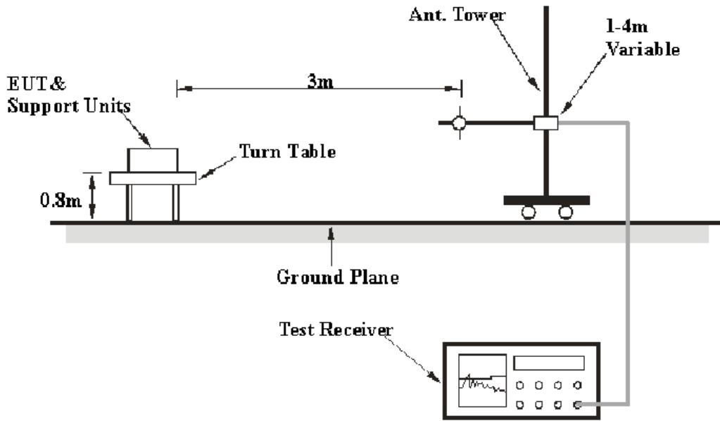
The radiated emission and out of band emission tests were performed in the 3 meters chamber test site, using the setup accordance with the ANSI C63.4-2009. The specification used was the FCC 15.209 and FCC 15.249 limits.
