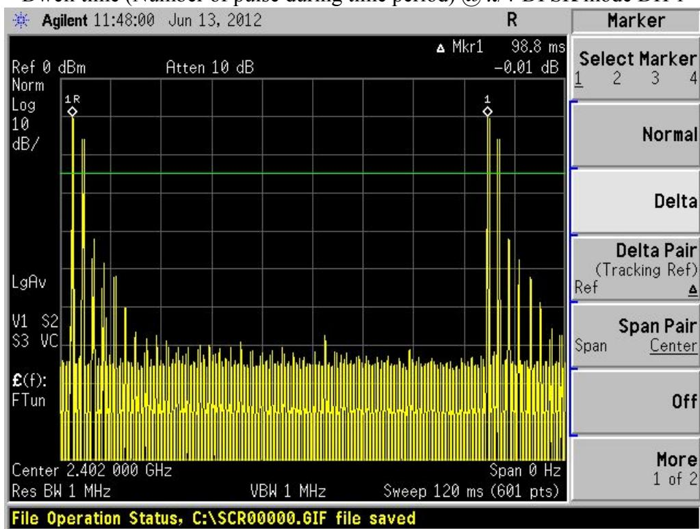
Dwell time (Single pulse) @  $\pi/4$ -DPSK mode DH 3
