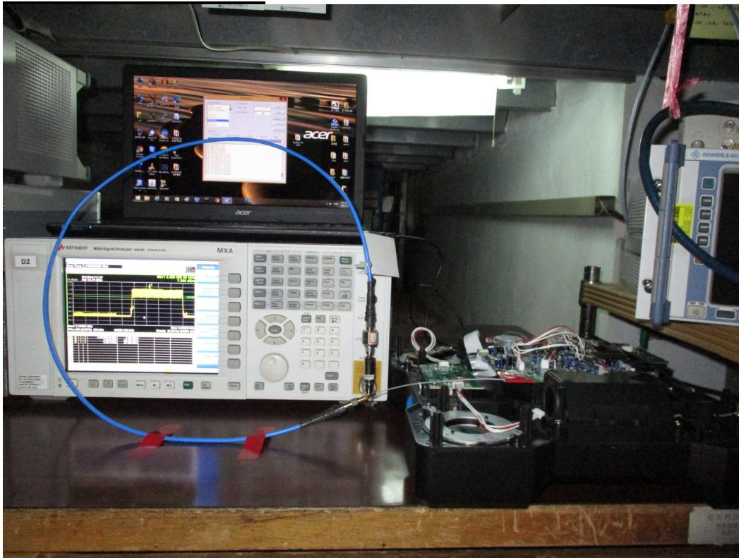
**CONDUCTED EMISSION MEASUREMENT SETUP****MODE: NORMAL OPERATION**
