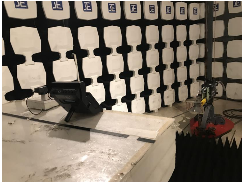
Measurement of Radiated Emission Test Set Up
