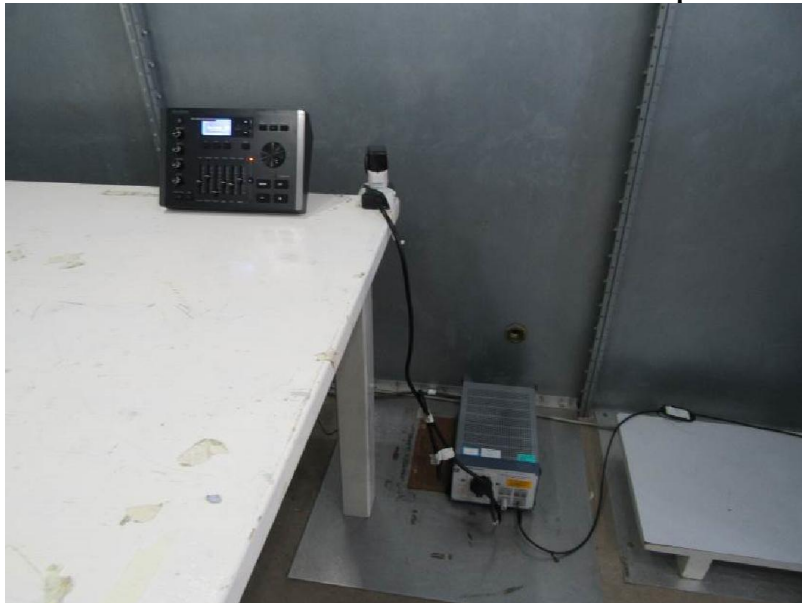
Measurement of Conducted Emission Test Set Up
