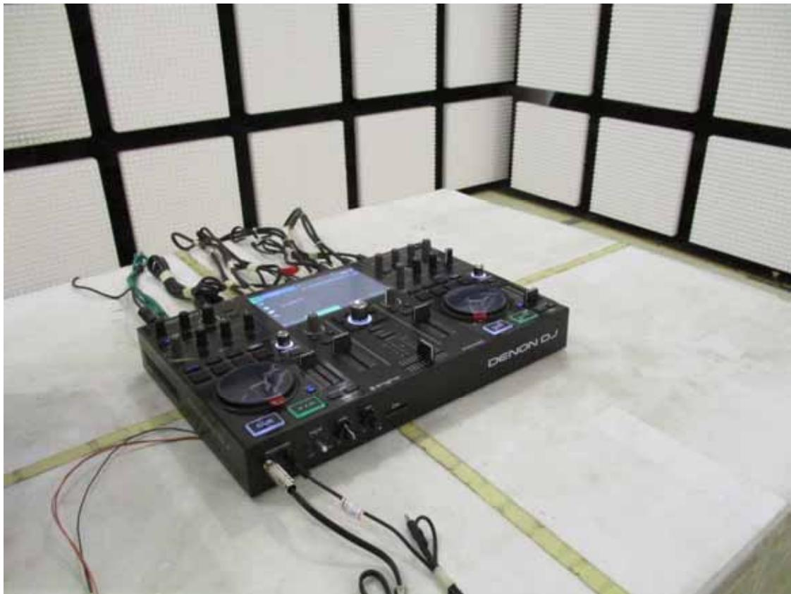
**RADIATED RF MEASUREMENT SETUP**
