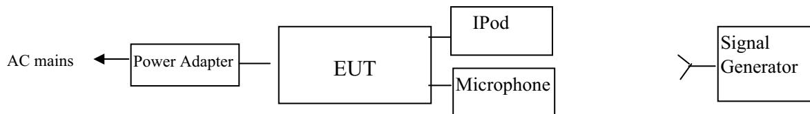
Test mode description: iPod playing 1 KHz sine audio signal and input to EUT by line in line, signal generator transmit 174.8MHz CW signal to EUT by an antenna in close proximity to the EUT, and the signal level was set sufficient to stabilize the local oscillator of the EUT.
