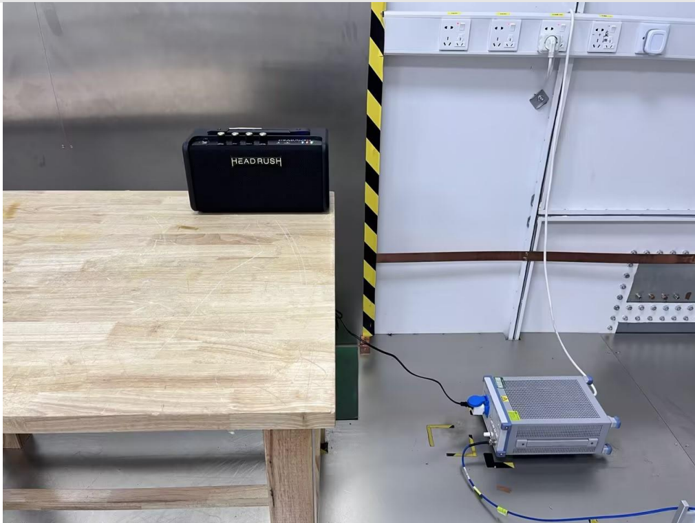
AC Power Line Conducted Emission
