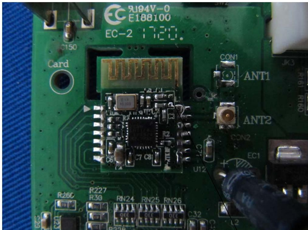
L1 chip inductor has been deleted, so the PCB antenna has not been used.
