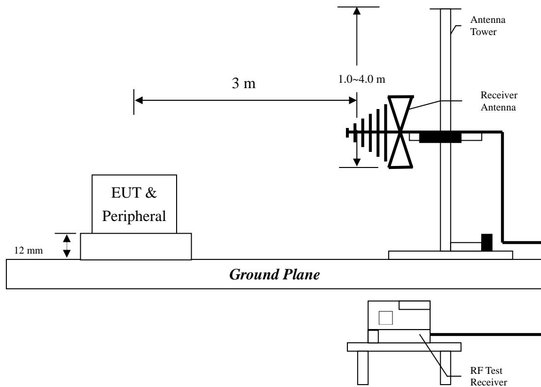
**Radiated emission above 1GHz uses Horn Antenna:**
