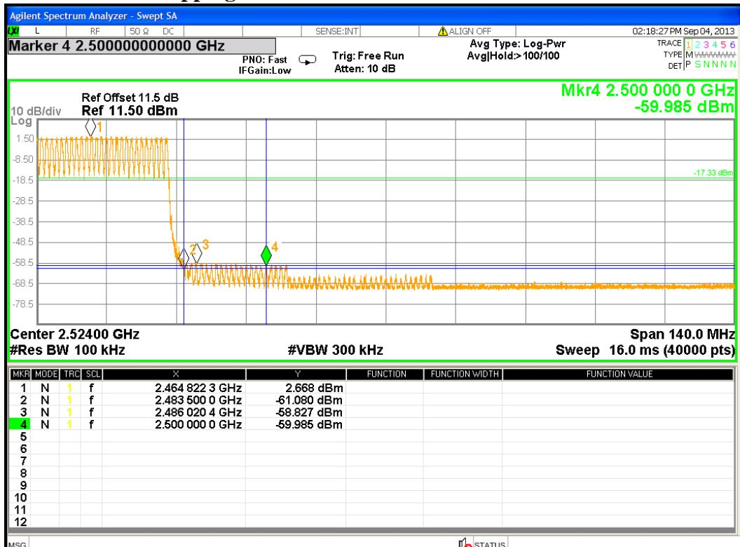
Hopping Enabled @ GFSK DH 5 channel 78 ~ 26.5 GHz
