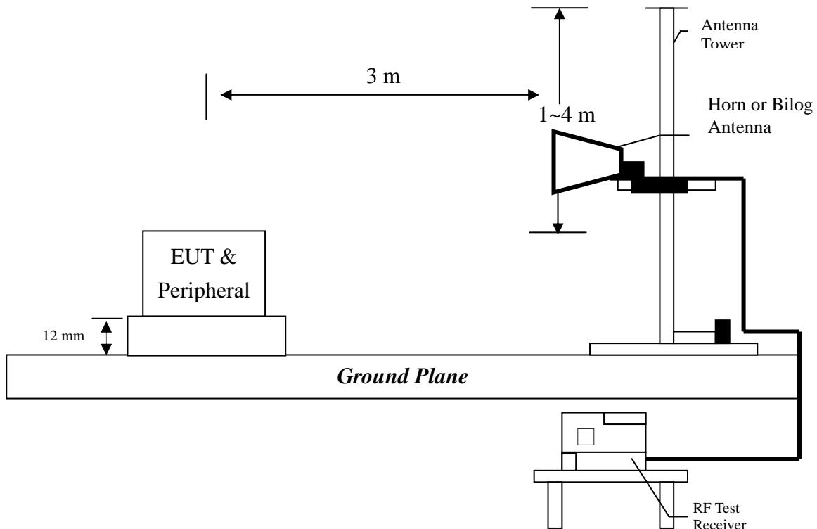
The signal is maximized through rotation and placement in the three orthogonal axes.
