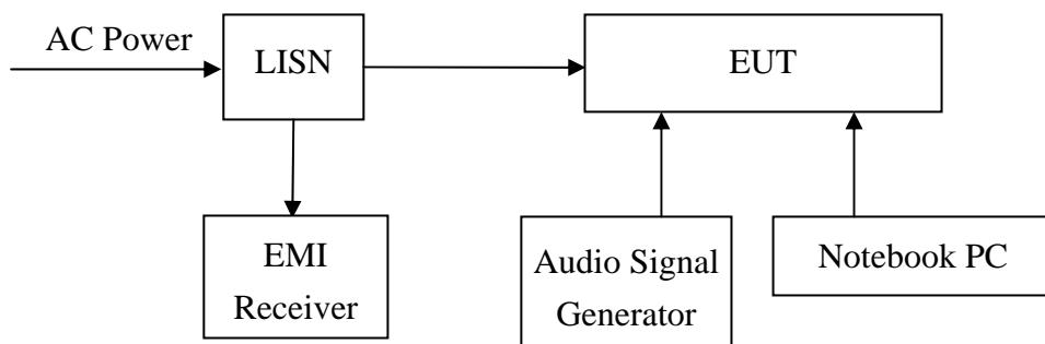
The test procedure was according to ANSI C63.4/2003.
