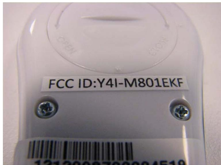
Label with **FCC ID:Y4I-M801EKF** is located at the rear side panel. The statement according to FCC part 15 §15.19(a)(3) is placed in User's Guide (Application exhibit User\_manual\_23370).
