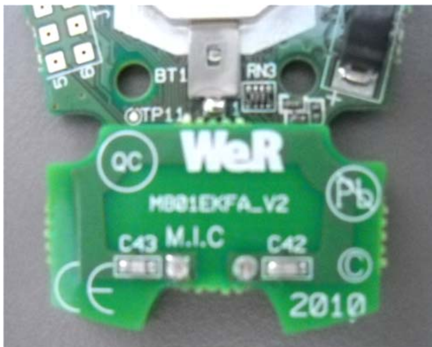
Photograph No.4 M801EKF wireless keyfob antenna
