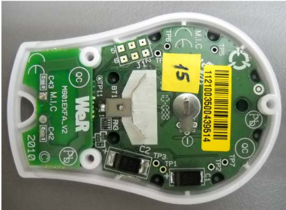
Photograph No.1 M801EKF wireless keyfob internal view
