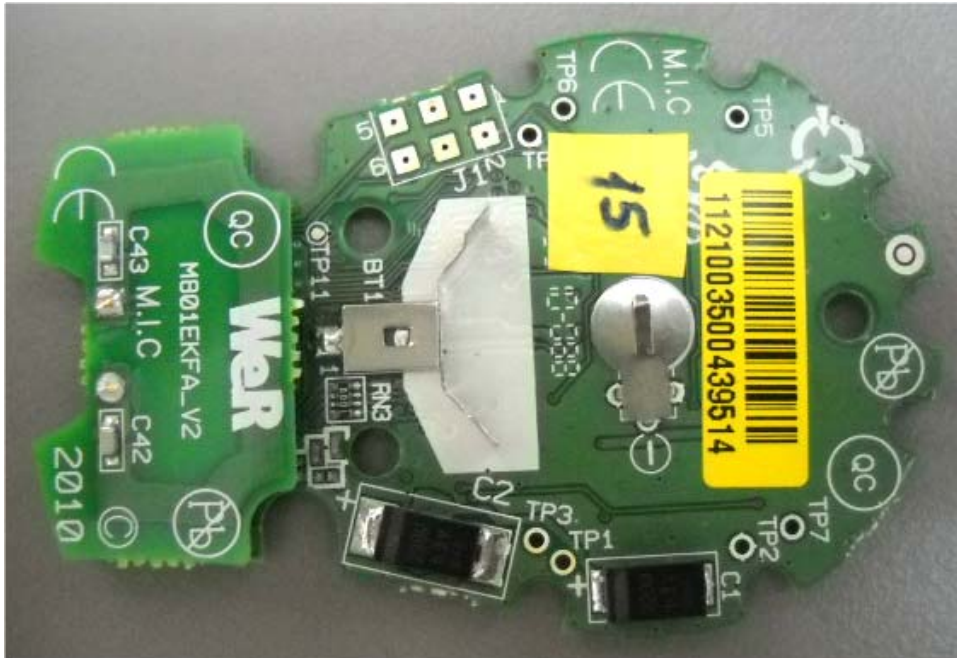
Photograph No.2 M801EKF wireless keyfob PCB front view
