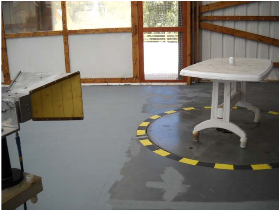
Photograph No.4 Setup for output power, OBW, spurious emission field strength measurements at the OATS in 1-18 GHz range
