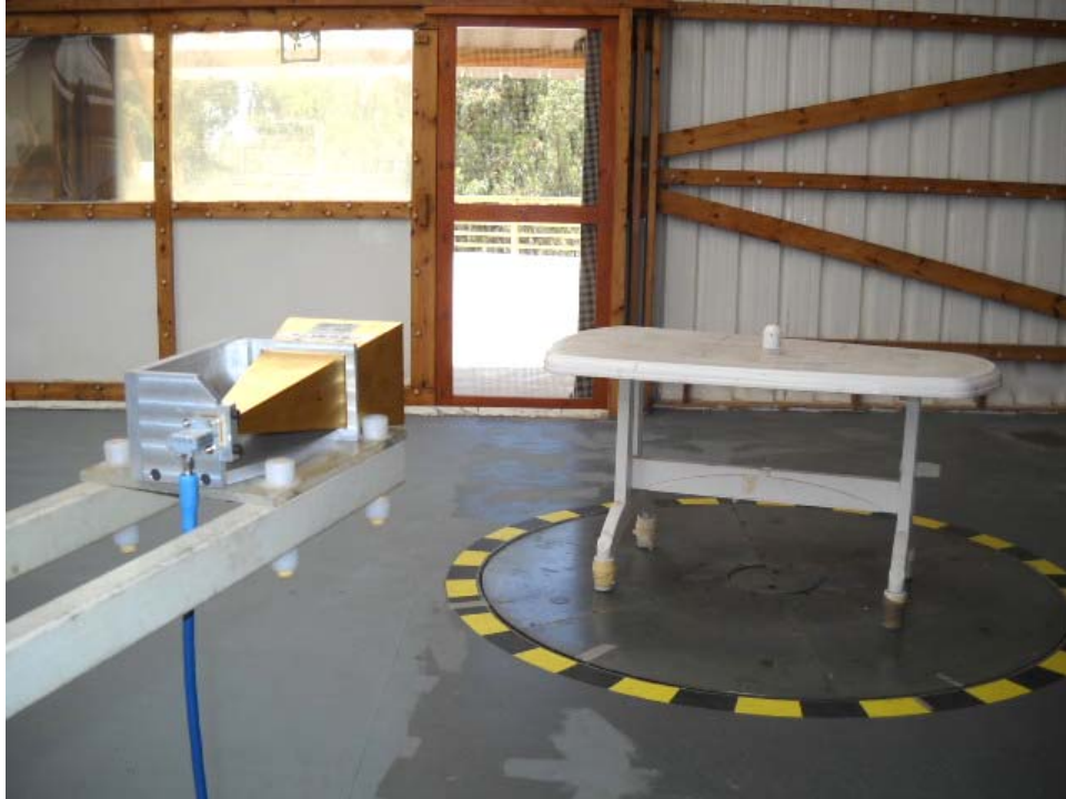
Photograph No.5 Setup for spurious emission field strength measurements at the OATS in 18 -25 GHz range
