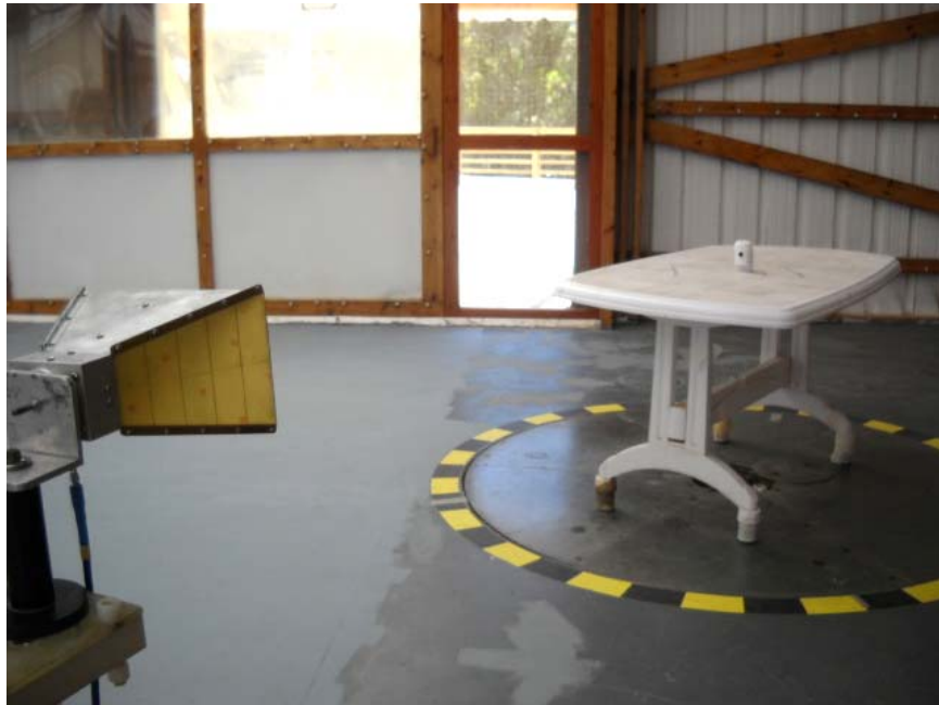
Photograph No.3 Setup for output power, OBW, spurious emission field strength measurements at the OATS in 1-18 GHz range
