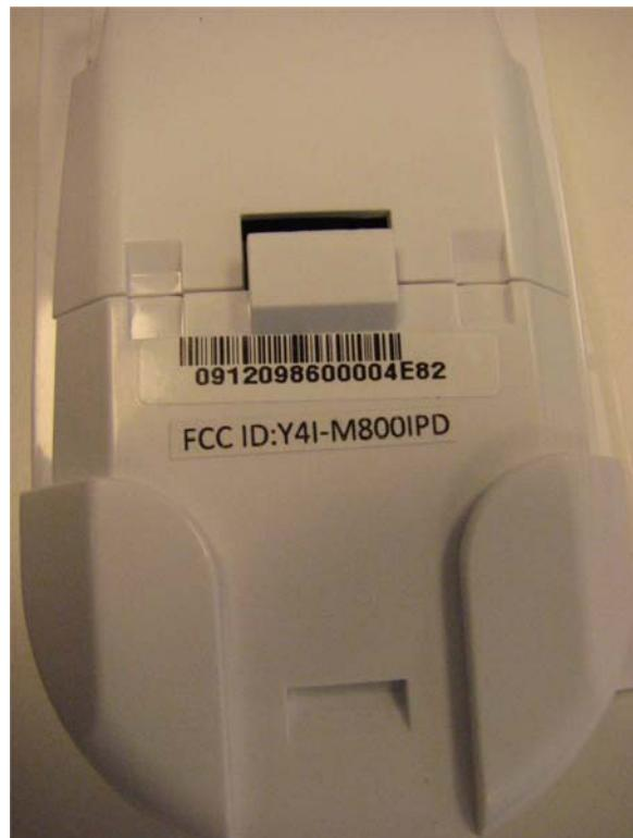
Label with **FCC ID:Y4I-M800IPD** is located at the rear side panel. The statement according to FCC part 15 §15.19(a)(3) is placed in User's Guide (Application exhibit User\_manual\_23369).
