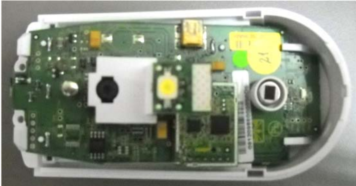
Photograph No.1 M800IPD indoor photo detector internal view
