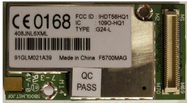
Bottom view of the internal GSM module.
