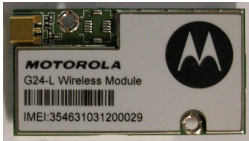
Top view of the internal GSM module.
