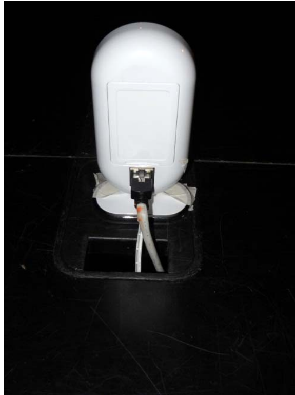
Photograph No.6 Setup for spurious emission measurements in the anechoic chamber, EUT close view
