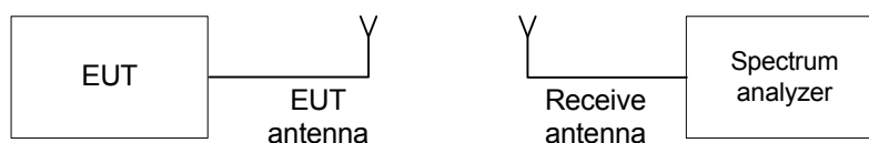
Figure 7.4.1 Occupied bandwidth test setup
