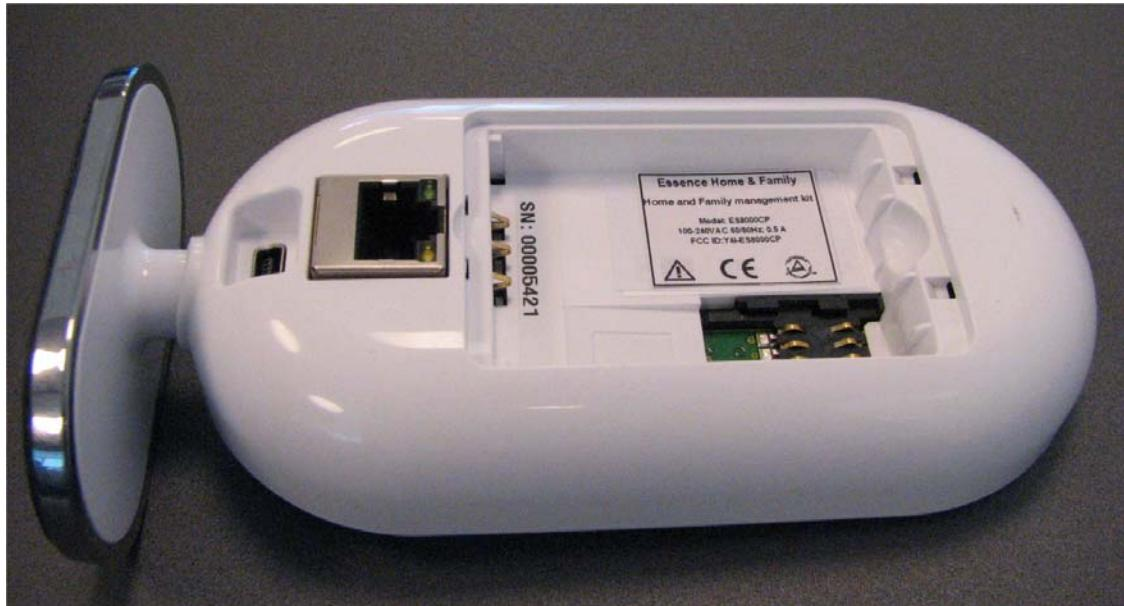
Label with **FCC ID:Y4I-ES8000CP** is located at the rear side panel in battery compartment. The statement according to FCC part 15 §15.19(a)(3) is placed in User's Guide (Application exhibit User\_manual\_23822).
