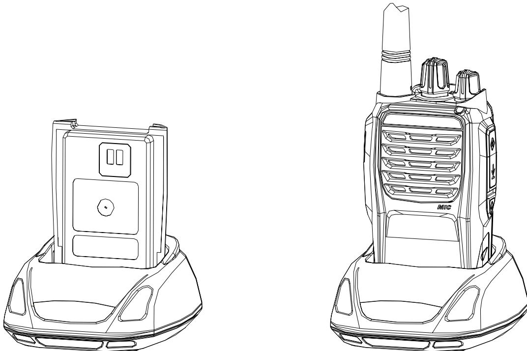
On the first charge, please leave the battery in that state of green indicator for 1~2 hours before you remove it from the charger to achieve the best performance of the battery. Then you can disconnect the power adapter from the AC outlet.
