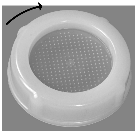
Figure 3-10: Screwing on the sampling grid
