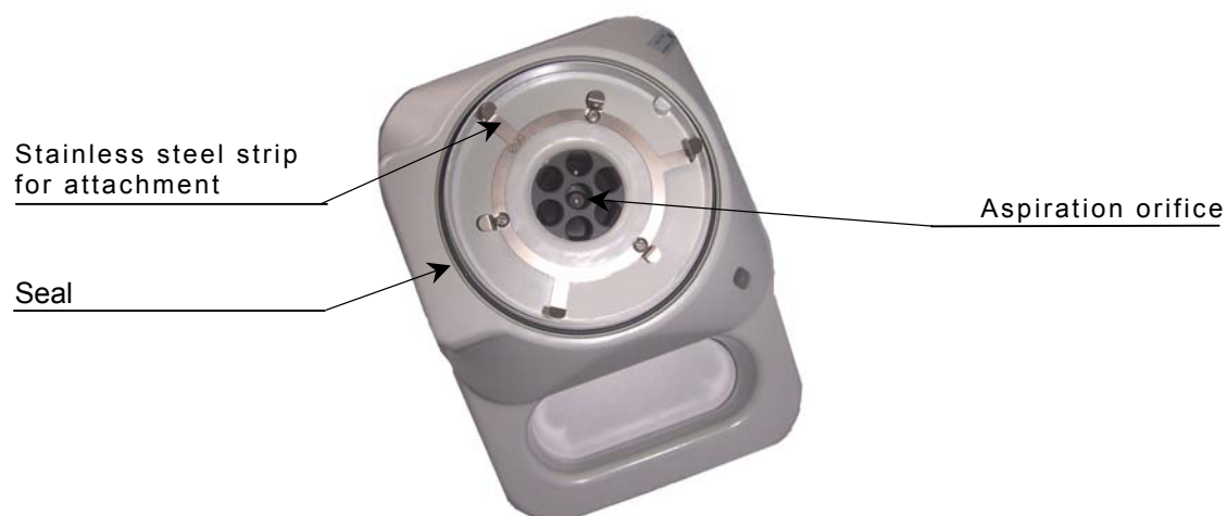
Figure 2-7: Sampling head and grid – 65, 70 or 90 mm Petri dishes
