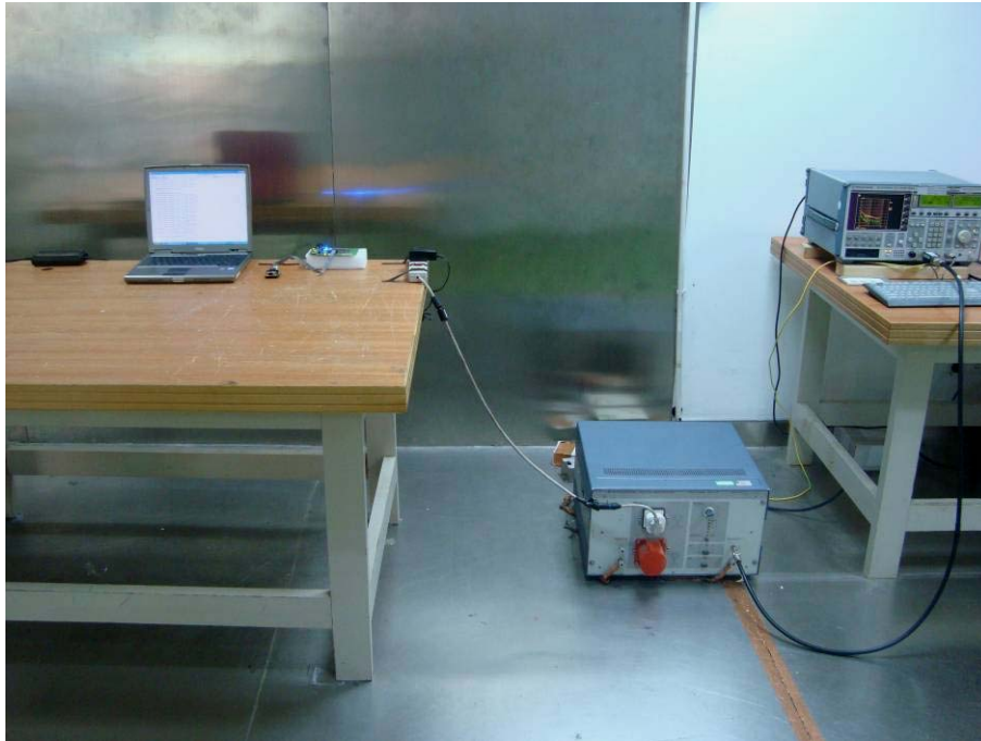
AC Line Conducted Emissions - Side View
