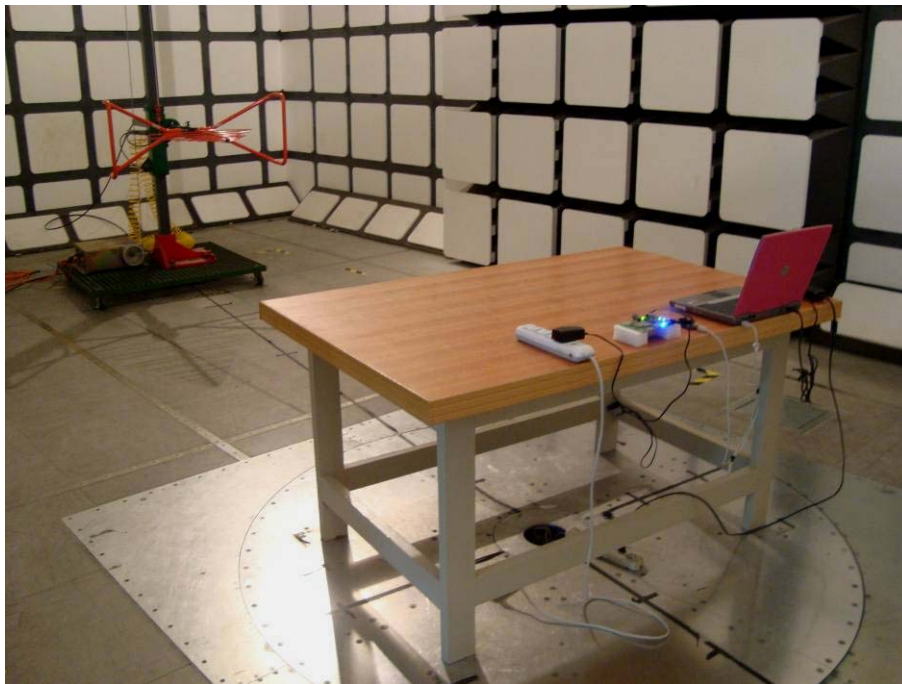
Spurious Radiated Emissions - Rear View
