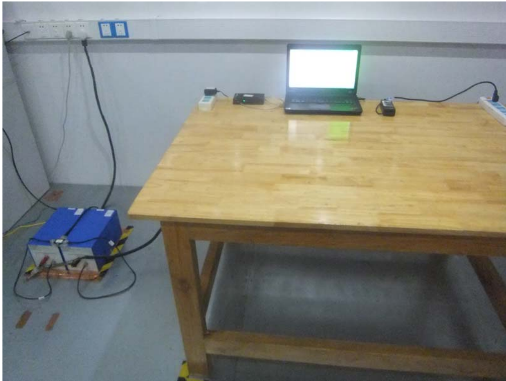
Conducted Emissions Test Setup Front View
