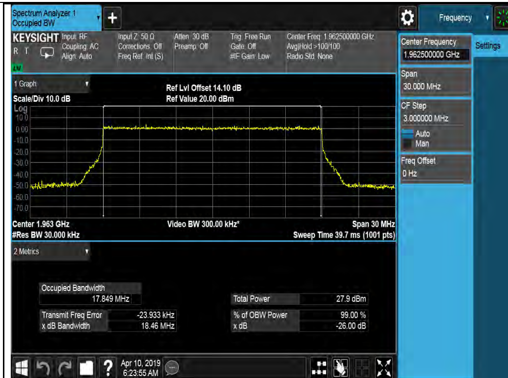
20M 64QAM Mid
