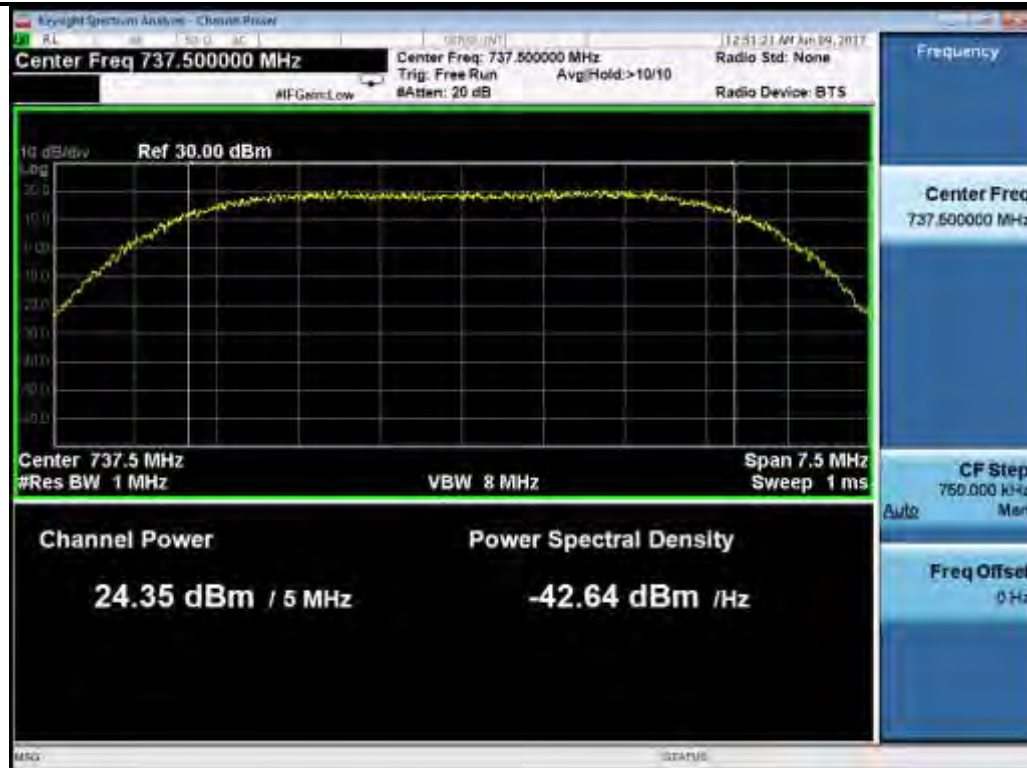
5M 64QAM Mid
