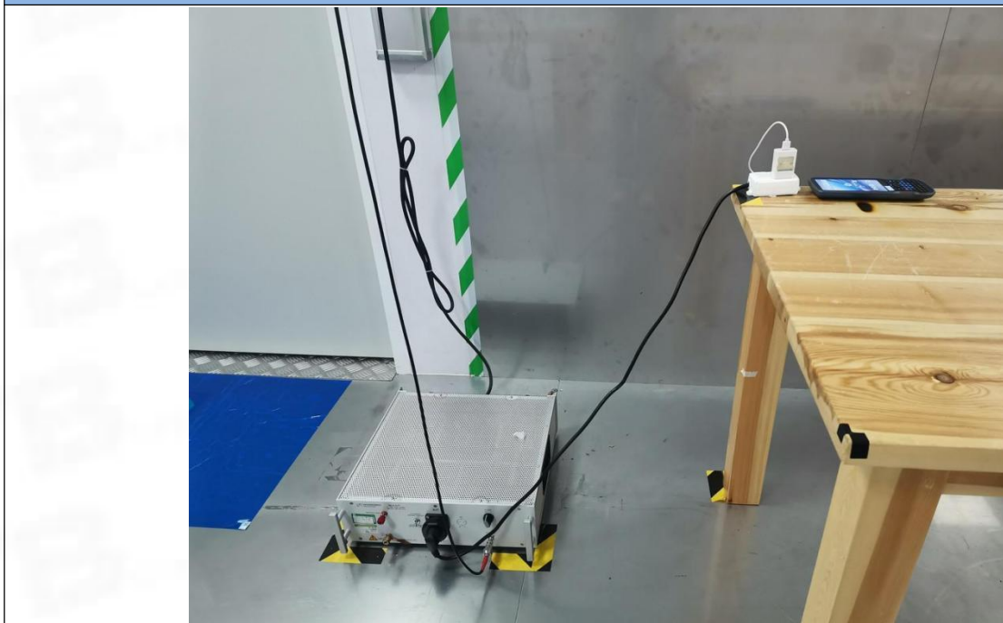
Conducted Emission at AC power line
