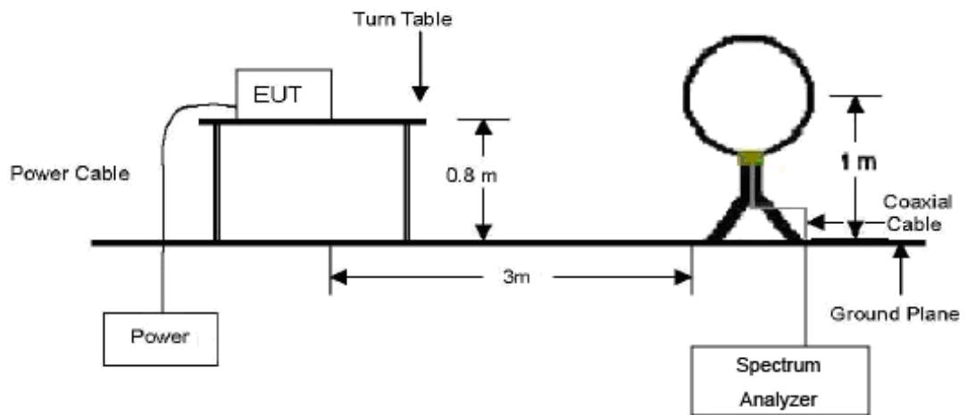
The diagram below shows the test setup that is utilized to make the measurements for emission from 30 MHz to 1 GHz Emissions.
